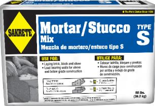
Sakrete® Type S Mortar/Stucco Mix is a preblended mixture of sand and masonry cement or sand, lime and portland cement. For laying brick, block and stone in load bearing walls and below grade applications. Build walls, planters, and chimneys. For tuck pointing or repairing existing mortar joints. Can also be used for scratch, brown and finish of walls. Meets property requirements of ASTM C270 and C1714.
